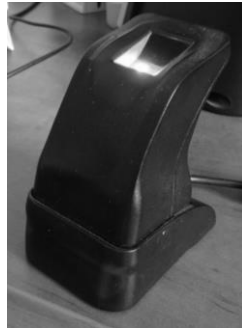
Figure 2 ZK4500 reader – optical sensor with 500 dpi resolution, sensing area 15 x 18 mm
