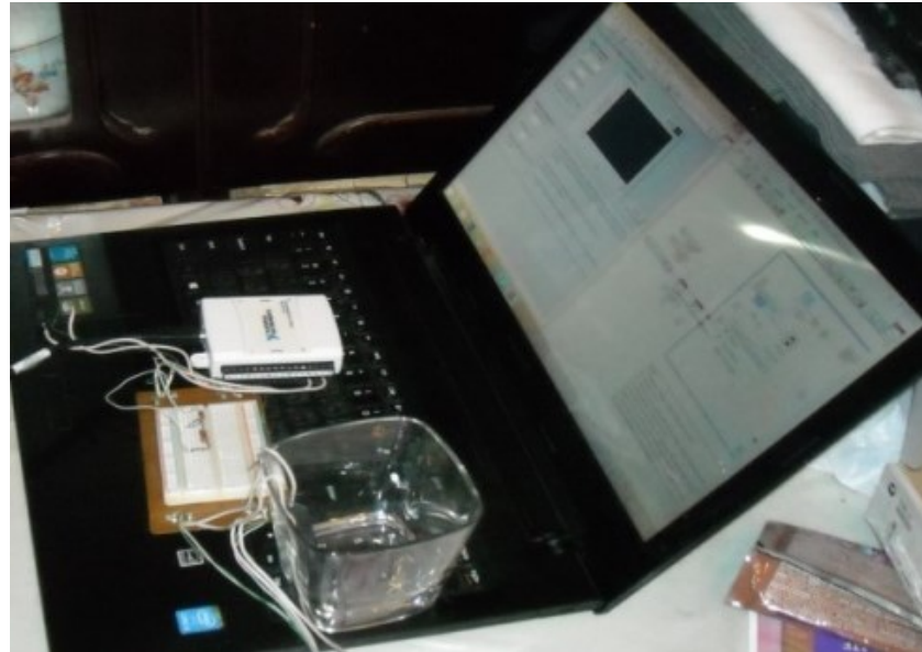
Figure 2 Virtual means of generating sinusoidal voltage and measuring the immittance of non-electric objects (juices), Source: own.
